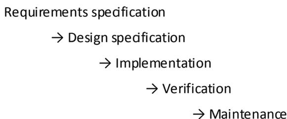
Its major disadvantage is that it is difficult to change requirements after the specification phase is completed.
